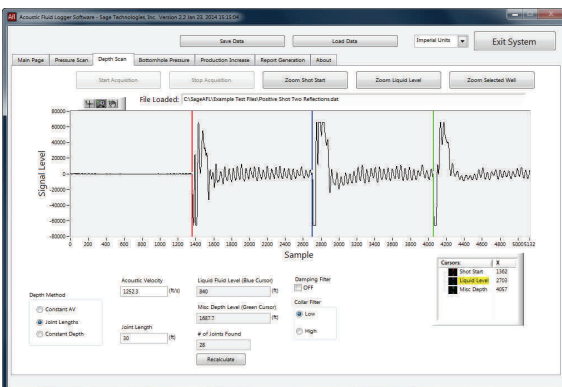
Sample Fluid Level shows compressed gas shot (red line), fluid level (blue), and second reflection of fluid (green).
