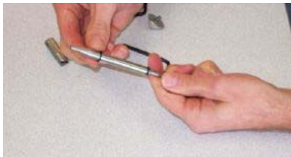
Photo 11, Attach tapered end of maintenance tool to shuttle, slide replacement o-rings onto shaft
