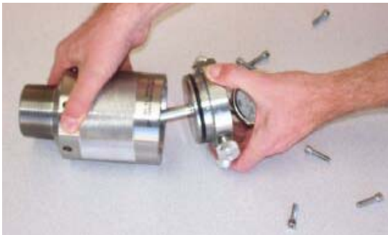
Photo 5, Separate top and bottom of gun
