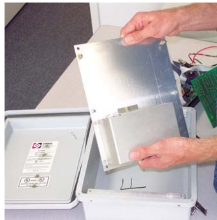
Photo 7, Remove battery plate from box
