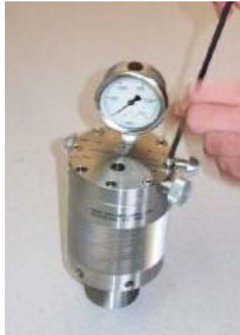
Photo 4, Loosen screws on top of gun
