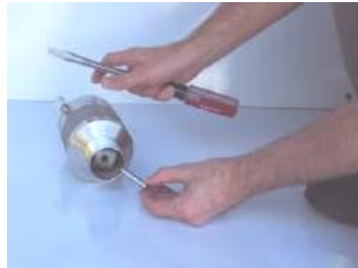
Photo 3, Remove retainer bolt
