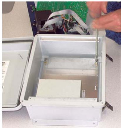
Photo 6, Remove bottom plate screws
