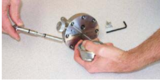
Photo 9, Remove shuttle valve from gun top
