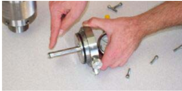
Photo 7, Replace small black O-ring on blast stem
