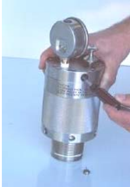
Photo 12, Remove fill valve cover to replace valve core
