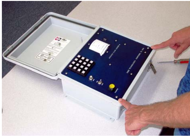
Photo 1, Remove front panel from Acoustic Fluid Logger
