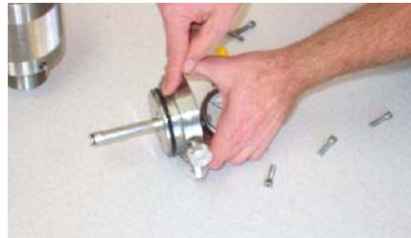
Photo 6, Replace large black O-ring on gun top
