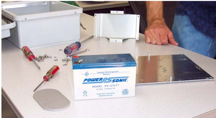
Photo 9, Replace with standard motorcycle battery, 12-volt, 7.0 amp
