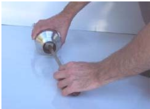
Photo 2, Loosen retainer bolt
