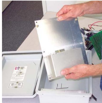
*Photo 7, Remove battery plate from box*
