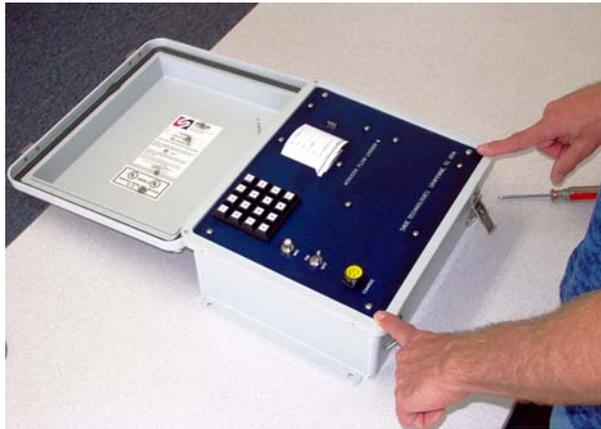
*Photo 1, Remove front panel from Acoustic Fluid Logger*
