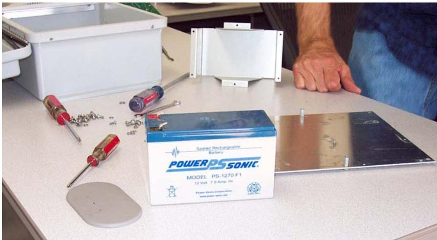
*Photo 9, Replace with standard motorcycle battery, 12-volt, 7.0 amp*
