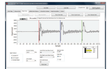
Above: Square Root of fluid level Amplitude Plot recorded with Acoustic Fluid Logger III. Right: Fluid level shot recorded with Acoustic Fluid Logger IV and Sage AFL software.
