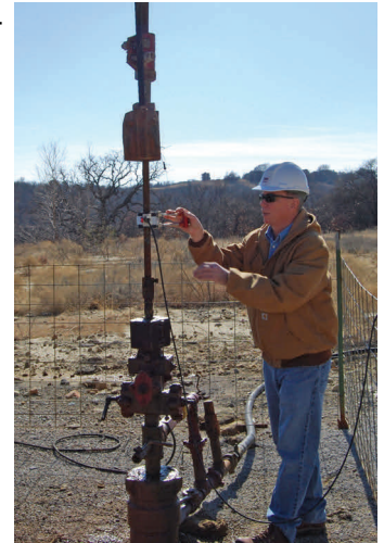
Installing Quick Clamp on rod string
